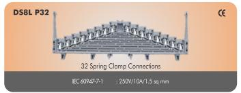
**DS8L:** DIN Rail Mounted Screwless Terminal Block having 8 Levels of feed-through connections. Used for marshaling applications where number of wires are very large. The construction of the terminal reduces the space requirement considerably in the panel. Available in two versions with the same terminal pitch for 8 inputs / 8 outputs and 16 inputs / 16 outputs.
